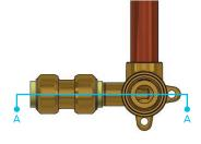
**TOP VIEW**PEX Fitting Attached
