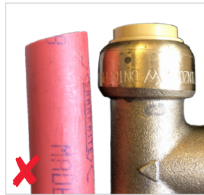
Pipe has not been cut square
