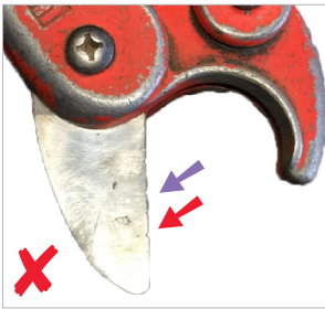
Cutting tool damaged
