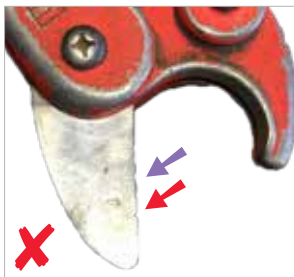
Cutting tool damaged
